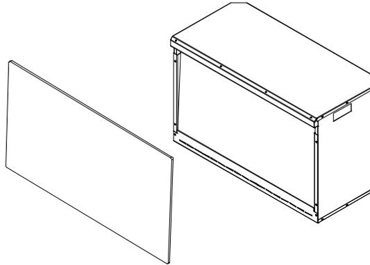
3. Pour the fire glass media into the tray. Feel free to use any combination of the fire glass media that you find most appealing. Insert the front glass panel back in place after the media installation has been completed.
