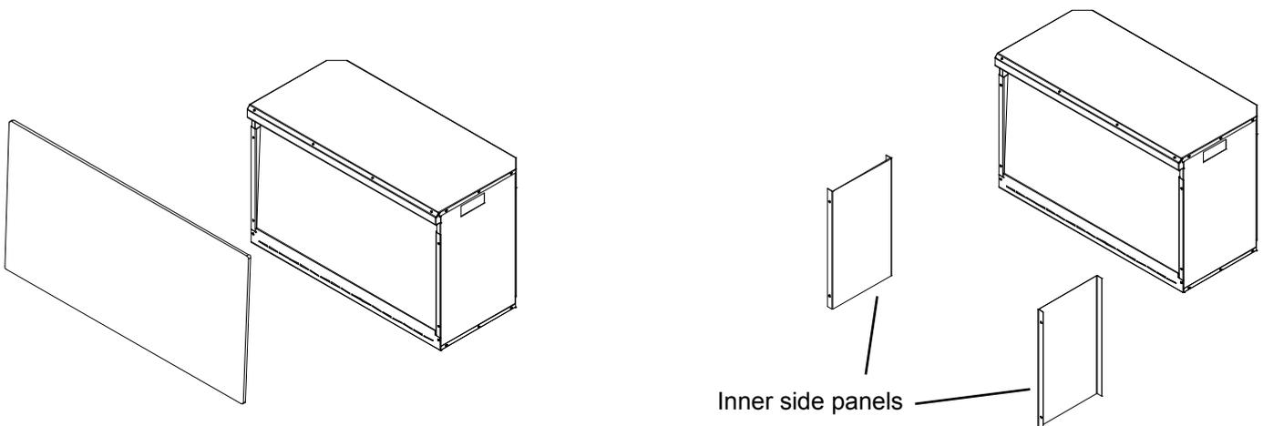
4. Put the trim back onto the appliance and fasten with screws. (NOTE: This step is to make sure that the fireplace fits the wall opening well and there is no gap between the trim and the wall after installation)
