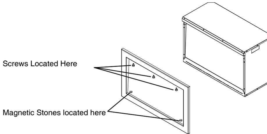
2. Carefully remove the front glass panel once the trim has been removed. Use caution as the glass is now loose.
