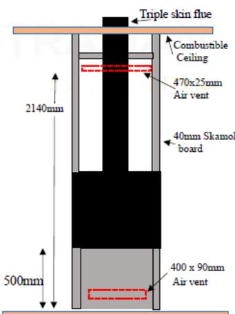
CLEARANCES BASED ON INSTALLATION HAWKWIND 200MM TRIPLE SKIN FLUE KIT. UNIT TO BE PLACED ON A BOX 1000MM[w] x 400MM[h] x 470MM[d] MADE FROM 50MM SKAMOL
